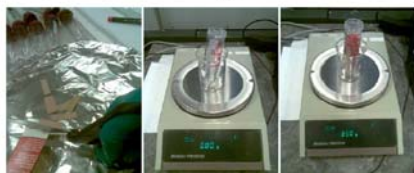
Figure 5.8 Double sided extraction of a food contact material: a) The sample is cut in strips b) the weight of the tube is recorded c) the weight of the paper is recorded.
